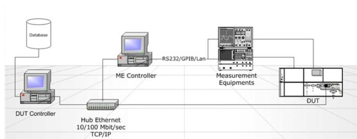
**Fig. 1** The Automatic Test System Architecture. **DUT** device under test, **DUT Controller**, **ME** Measuring Equipments which collect and check observable values from the DUT, the ME Controller connected with the ME
